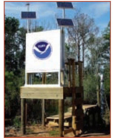
New tidal station surveyed in at Weeks Bay to provide most accurate real time monitoring information.
